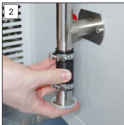
2. Slide the hose including the second hose clamp D32 over the outlet pipe below.
