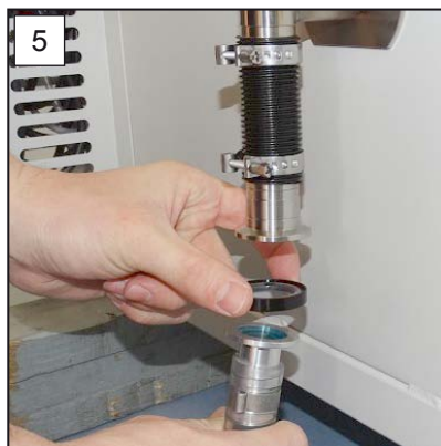
5. Place the centering ring between the flanges of hose nipple and your exhaust connection.
