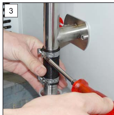
3. Fix the hose piece at the outlet pipe with the hose clamp; Phillips screwdriver size 2.
