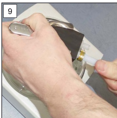
9. Slide the vacuum hoses onto the hose nozzles at the plug.
